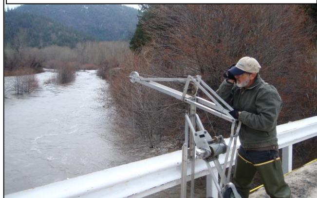
Terry Benoit, CRM Project Mgr., measuring high flows on Indian Creek at Fournoy Bridge, March 16, 2011
