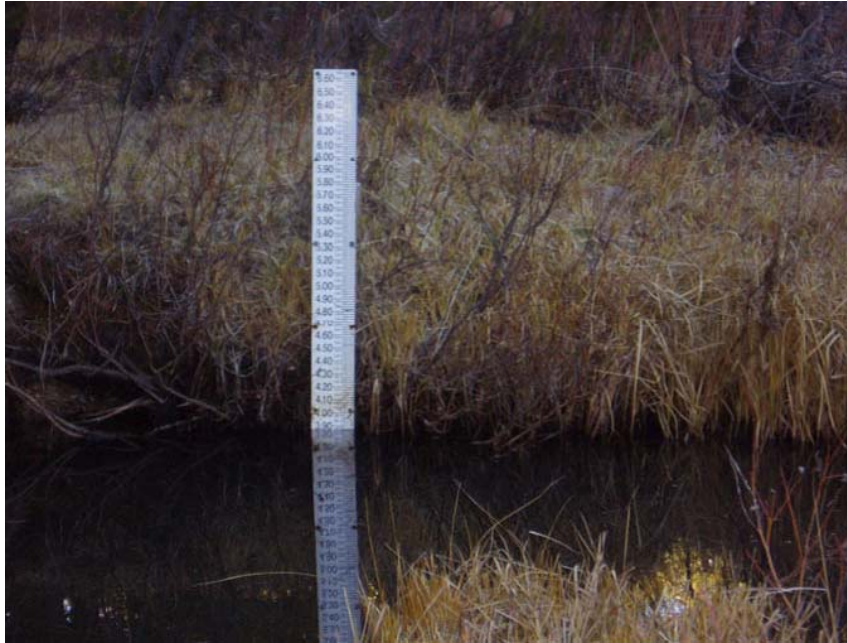
Photo 7. Staff gage used to measure stage of Big Meadows Creek (Date: Nov 7, 2007).
