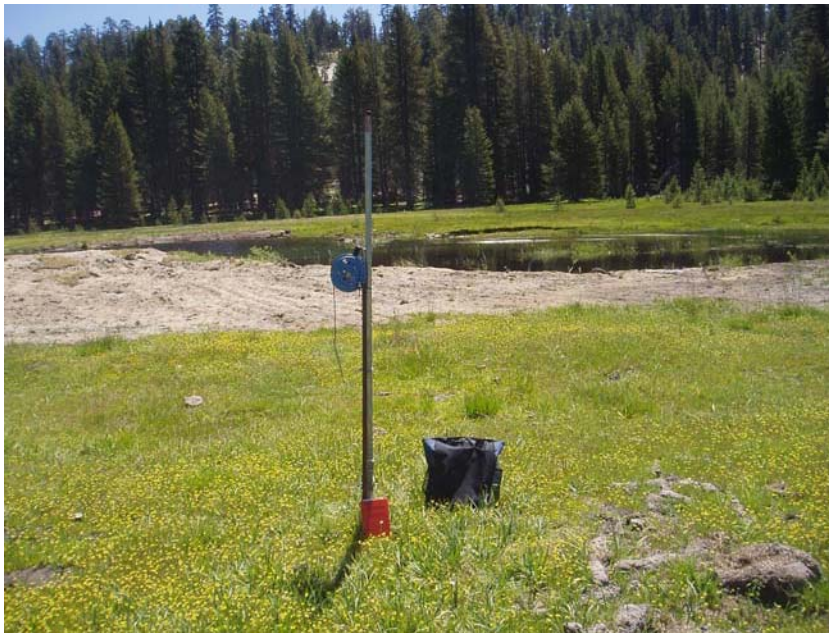
Photo 8. Middle piezometer (Reach B2) showing electric sounding device used to measure groundwater levels. Photo looking toward right bank with pond in background (Date: July 5, 2008).
